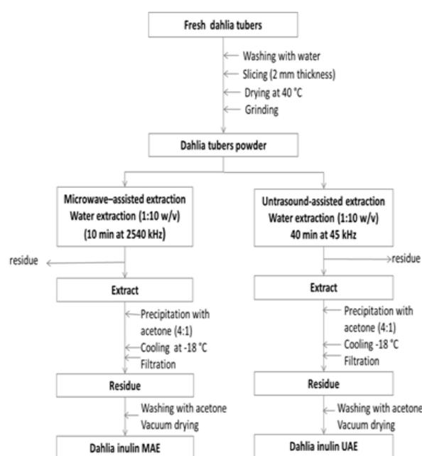
Figure 1. Schematic procedure for MAE and UAE of inulin from dahlia tubers
